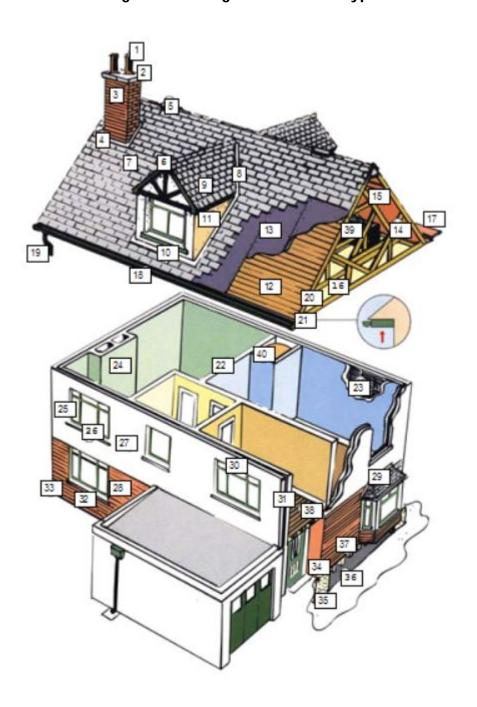
Dormer flashing 10 Dormer cheeks 11 12 Sarking Roof felt 13 Trusses 14 15 Collar 16 Insulation 17 Parapet gutter Eaves guttering 18 Rainwater downpipe 19 20 Verge boards / skews 21 Soffit boards 22 Partition wall Lath / plaster 23 24 Chimney breast 25 Window pointing Window sills 26 Rendering 27 Brickwork / pointing 28 Bay window 29 30 Lintels 31 Cavity walls / wall ties
