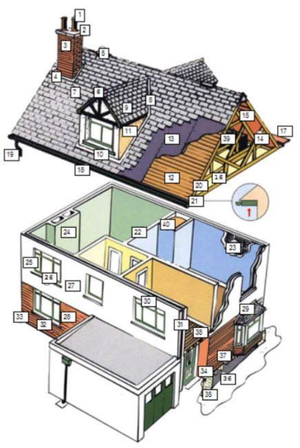
3 Chimney head Flashing 4 Ridge ventilation 5 Ridge board Slates/tiles 8 Valley guttering 9 Dormer projection Dormer flashing 10 Dormer cheeks 11 12 Sarking Roof felt 13 Trusses 14 15 Collar 16 Insulation 17 Parapet gutter Eaves guttering 18 Rainwater downpipe 19 20 Verge boards / skews 21 Soffit boards 22 Partition wall Lath / plaster 23
